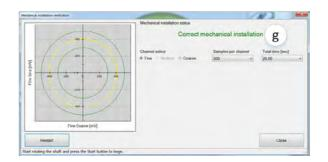
(h) If the SW indicates "Incorrect Mechanical Installation," correct the mechanical position of the rotor, as presented in paragraph 3.3 - "Rotor Relative Position."
