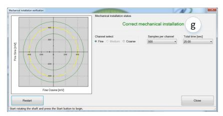
(h) If SW indicates "Incorrect Mechanical Installation," place the mechanical shims below the rotor, as presented in paragraph 3.3 - "Rotor Relative Position."
