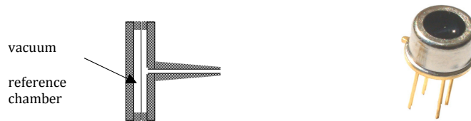
Fig 3, Principle of the absolute pressure sensor.
