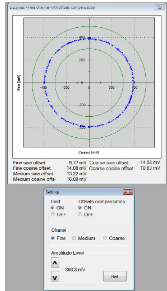
In case the reading data (blue dots) are not evenly distributed on a thin circle, you may experience "noise" in your installation (check shaft/stator grounding).
