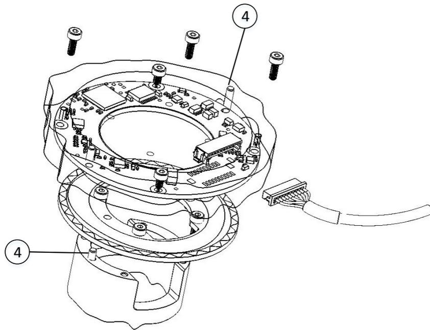
Encoder Stator / Rotor relative position
